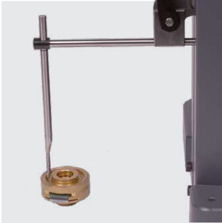
Depth measurement with accessories 930-2108 and 930-2105
