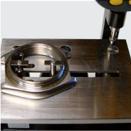
Internal measurement in 2 – points with auto-centering of the part on LVS 50
