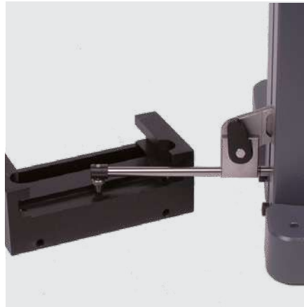
Depth measurement with accessories 930-2108 and 905-2204
