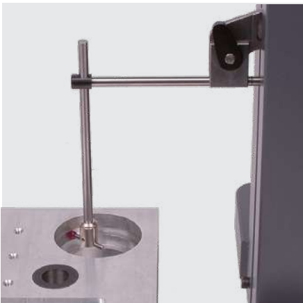
Internal groove measurement with accessories 930-2108, 930-2110 and 905-2207
