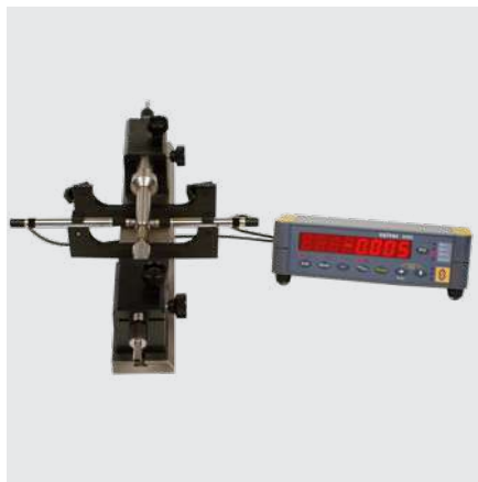
P5 probes connected to a D50S unit measuring the external diameter of a shaft
